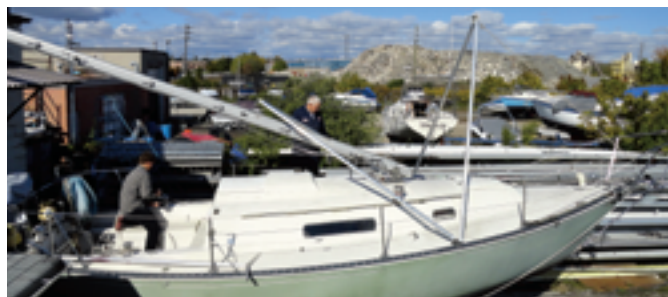
Two A-frames share common pivot points at the deck and are connected by a wire between their apexes. The forward one provides the raising lever and the after one lateral support for the mast.
